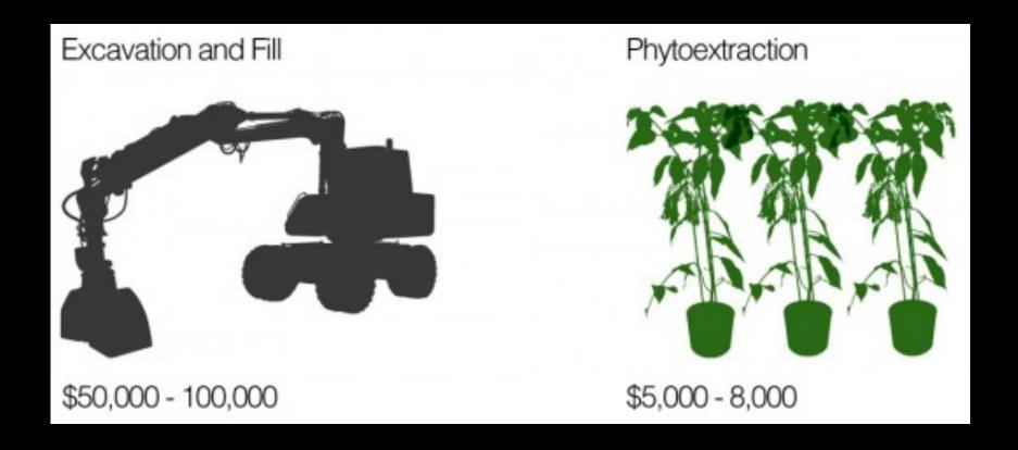
The costs associated with remediating lead contamination on a 2,500sf lot through phytoextraction using Indian Mustard can be reduced to 10% of the cost of excavation and fill.
